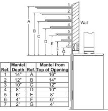
Figure 6 - Clearances for Combustible Mantels
